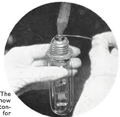
(4) The alignment of the filament is now made by projecting the filament image on to a screen marked out for correct positioning.
