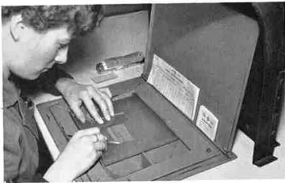
(2) Every filament is thoroughly inspected in the manner shown above before being used.
