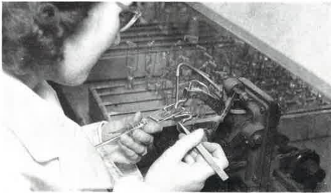
(2) The filaments are now mounted, with great accuracy, onto their supports by the spot-welding process.
