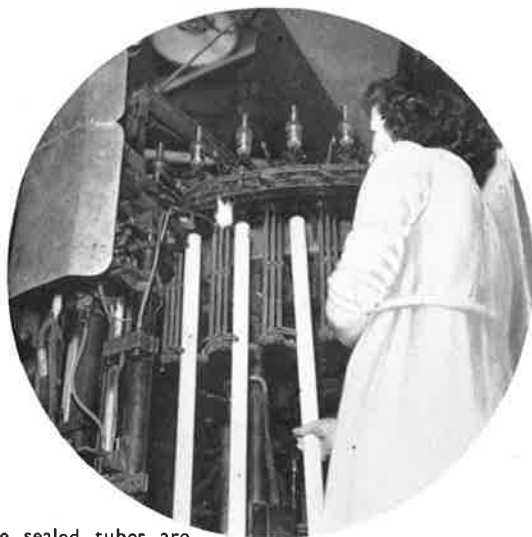
(3) The sealed tubes are now capped — either B.C. or bi-pin.
