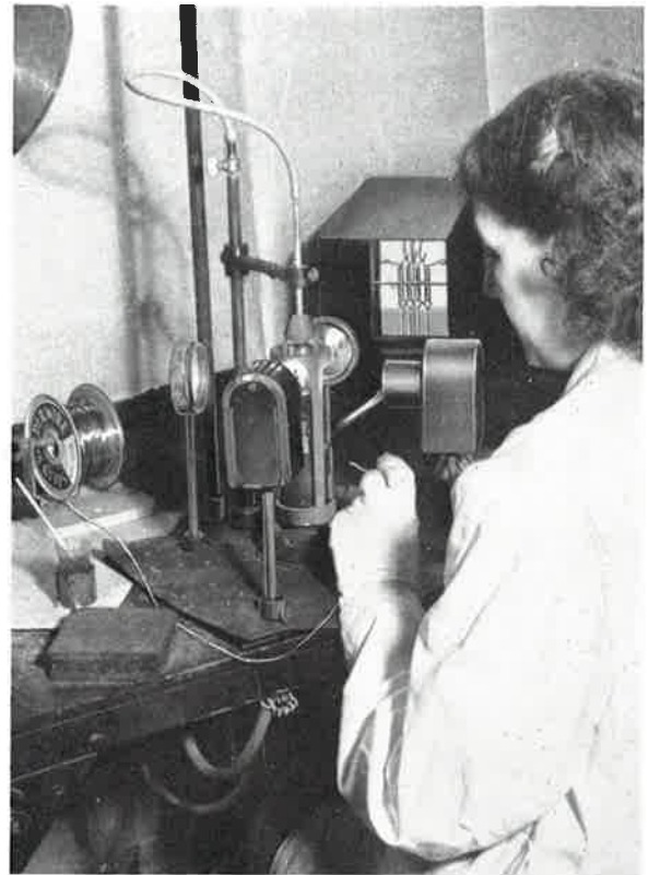
(4) The alignment of the filament is now made by projecting the filament image on to a screen marked out for correct positioning.
