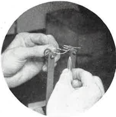
(1) The filaments having been wound are shaped over a heated element, great care being taken to ensure correct filament area.
