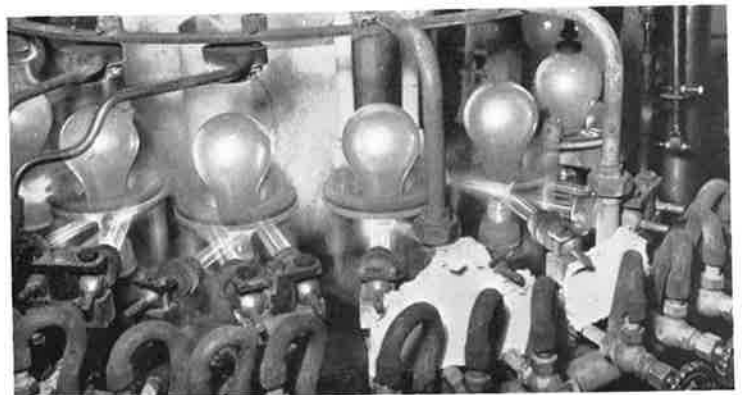
(5) A close-up of the sealing process — Mazda precision ensures perfect standardization of each product.
