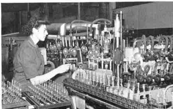
(4) The mounted filaments are inserted into glass envelopes which are then sealed, carefully heated, and shaped into the familiar "bulbs."
