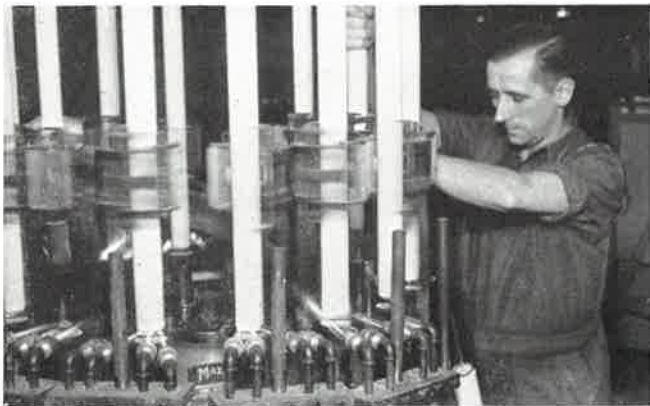
(2) Cathodes are then inserted into each end of the tube, which is subsequently sealed in the manner shown above.
